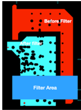
Figure 44 This layout means strong coupling between the two traces (trace before and after the filter)
